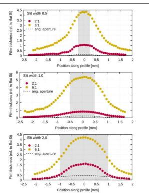
**Fig. 1**. Deposition thickness profiles in cavities with slit openings 0.5, 1.0 and 2.0 mm normalized to the film thickness on the flat Si. The data obtained by ellipsometry for  $CO_2:C_2H_4 = 2:1$  and 6:1 are compared to the thickness profile that is theoretically expected by a geometrical shielding of thermalized particles depicted as a view angle at a given point (``angular aperture"). The slit widths are shown as shaded areas.
